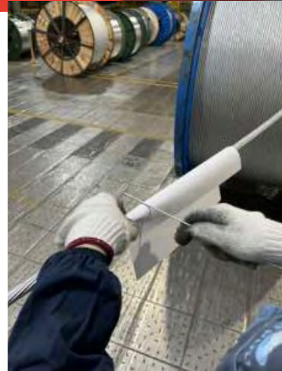
Lay length testing
